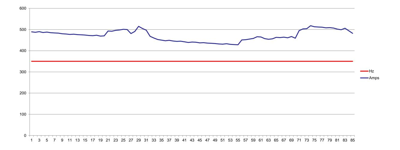
The graph above shows the current drawn by the pump on the initial test run, with operation at constant speed (35Hz output frequency). The time period of the test data is approximately 4 minutes, and shows the pump current drawn to be a minimum of 42.8 Amps, maximum 51.3 Amps, average 47 Amps.
