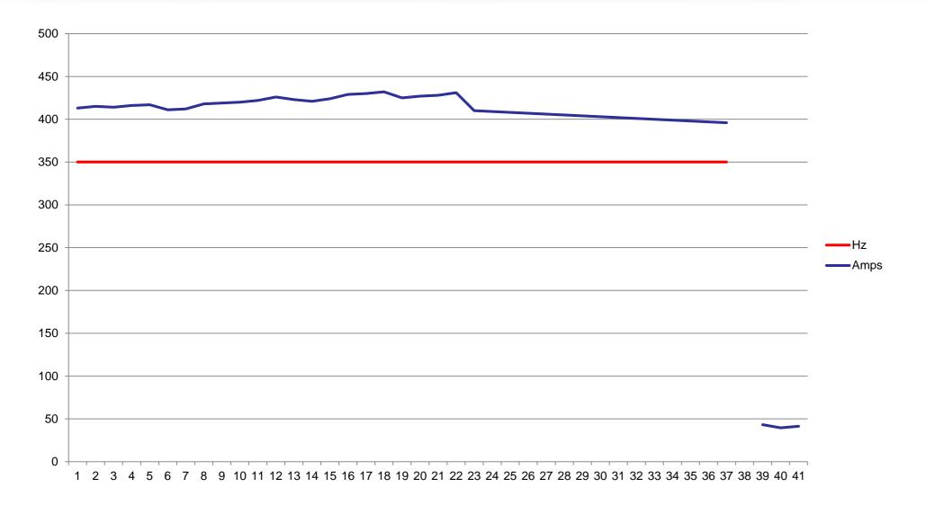
Same pump at the same speed after cleaning, the output current was much more stable, varying only from a minimum of 39.6 Amps, Maximum 43.2 Amps, Average 41.3 Amps. The clean impellor of the pump is considerably more efficient, as displayed by the reduced running current, which represents an energy saving of 12% achieved in this case.
